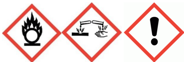
Flame over circle Corrosion Exclamation mark
